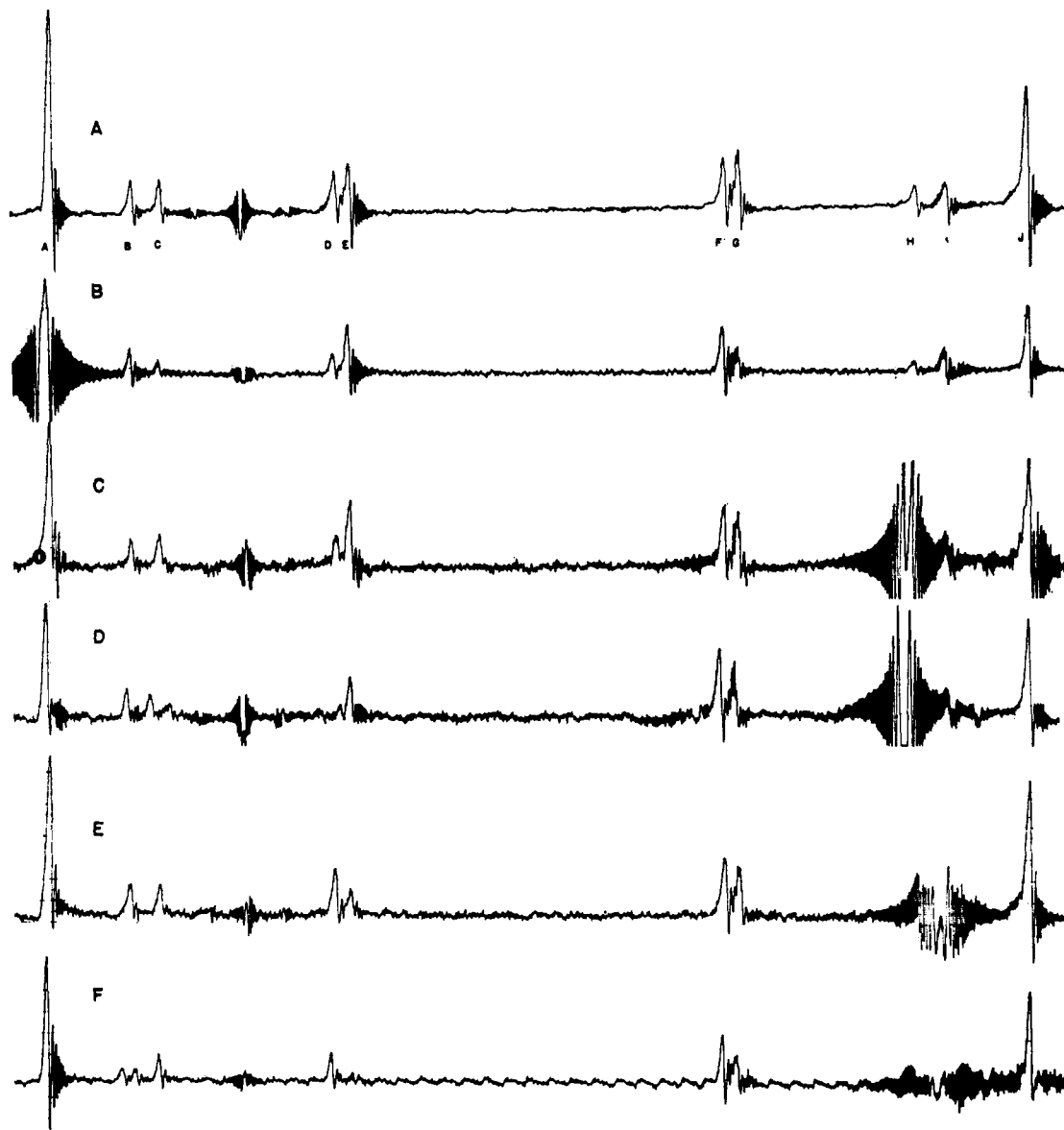
Fig. 1.—Frequency sweep n.m.r. spectra of cis -CHFCHF in \text{CCl}_3\text{F} at 60.0 Mc.: (A) single resonance spectrum, and double resonance spectra with strong irradiation at (B) line a, (C–D) line h and (E–F) line i.
